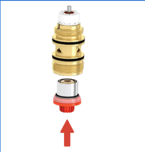
Step 6: put back the diaphragm. Push it in its seat
