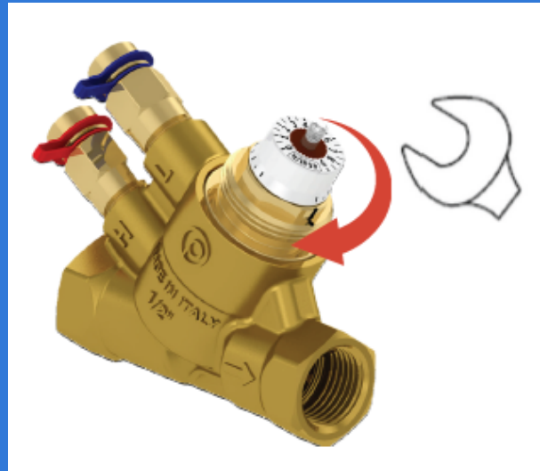
Step 8: screw the headwork with 20 Nm torque
