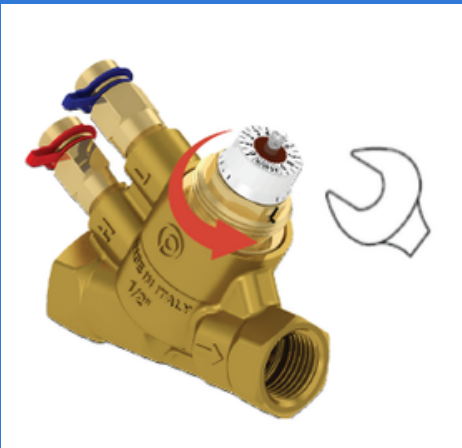
Step 2: using a 21mm spanner unscrew the headwork.
