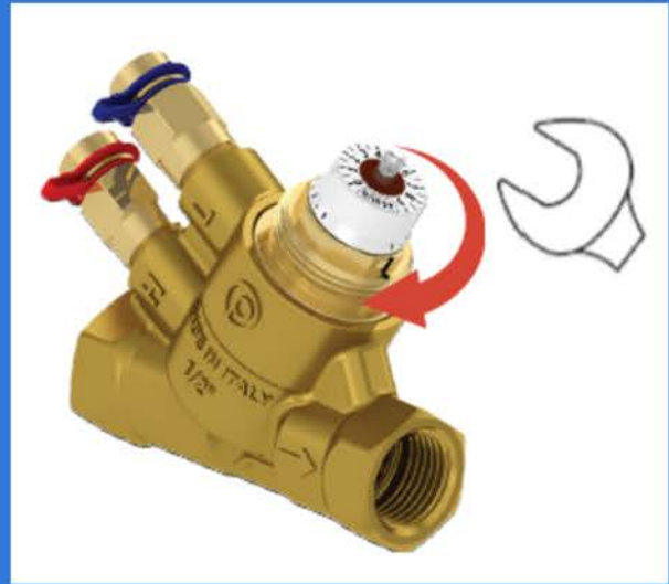
Step 8: screw the headwork with 20 Nm torque
