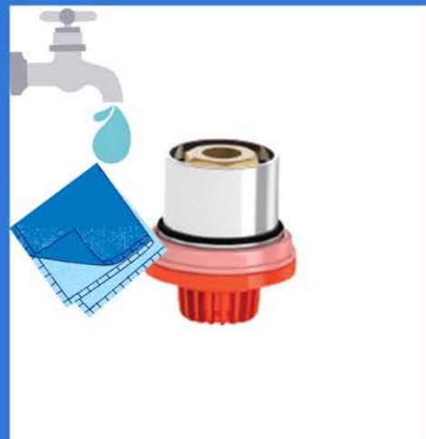
Step 5: clean the diaphragm with water and a cloth
