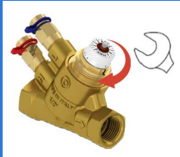
Step 8: screw the headwork with 20 Nm torque
