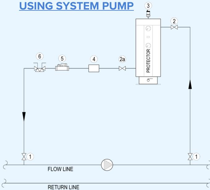
Protector keeps your system clean by adapting to your needs. Two different filtering elements, completely interchangeable, remove suspended particles from the recirculating system.
