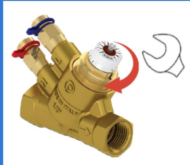
Step 8: screw the headwork with 20 Nm torque
