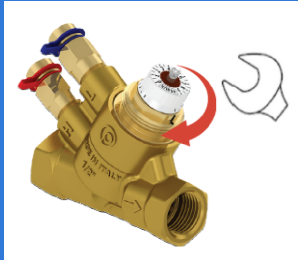
Step 8: screw the headwork with 20 Nm torque
